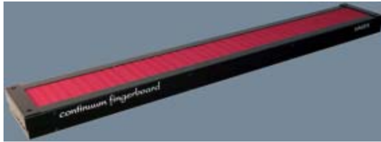
Figure 5 – The Haken Continuum Fingerboard
