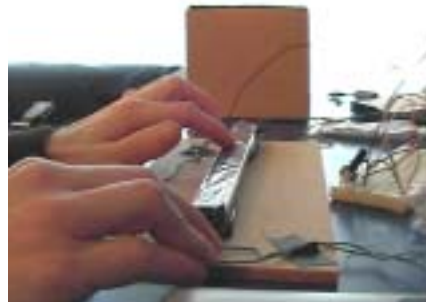
Figure 11 – Showing the use of each hand for controlling pitch (pressure) and volume (position)
