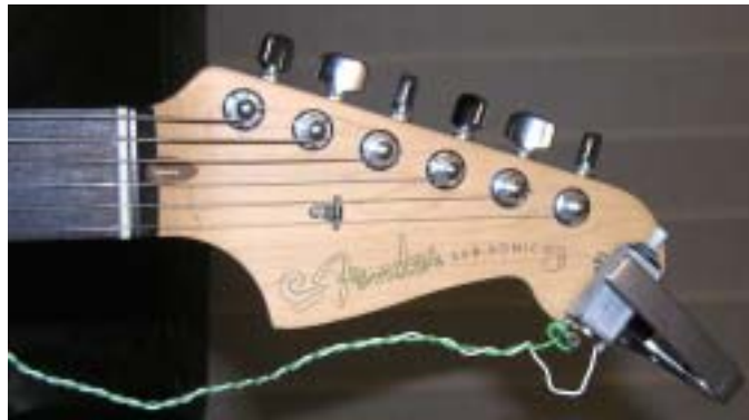
Figure 18 – Using a motor as a speaker, sending vibrations through a solid object
