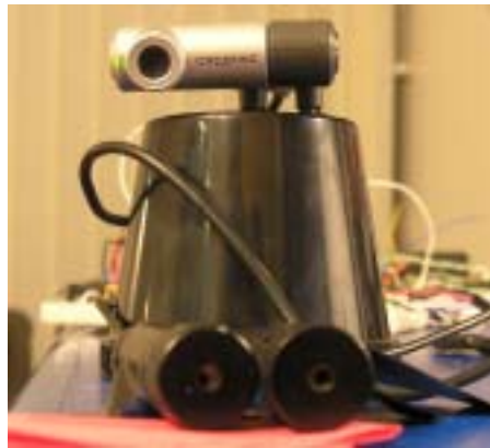
Figure 22 –Webcam and laser pointers as a distance measurer
