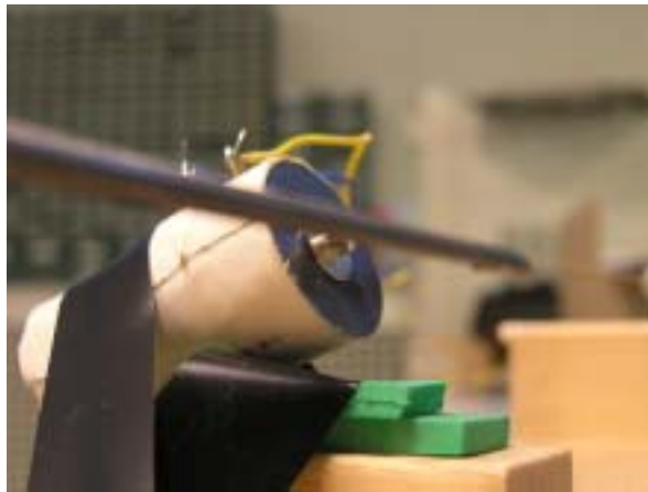
Figure 17 – Using a solenoid to vibrate the metal rod.
