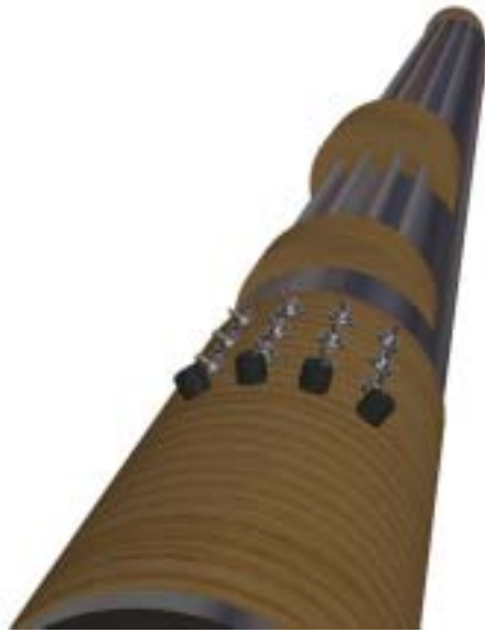
Figure 28 – Switches for setting playing modes, and volume knobs for each rod
